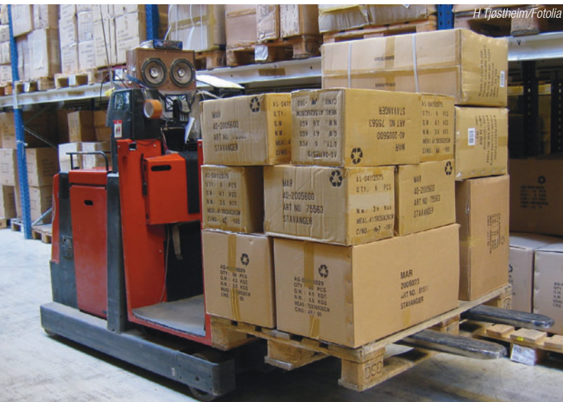
Electrical machinery in modern warehouses is a potential source of ignition
